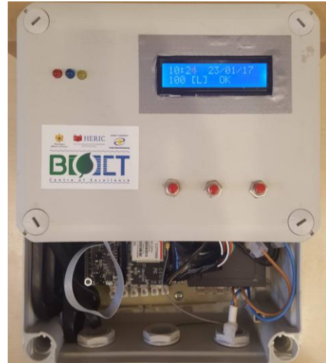
Fig. 5. Prototype of the smart irrigation system
