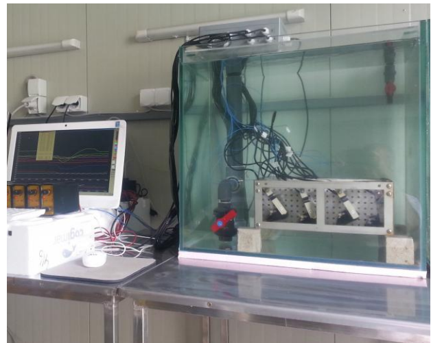
Fig. 4. The measurement of mussels valve movements
